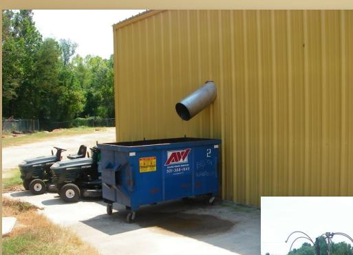
Dumpsters must either be covered or drain back to treatment
